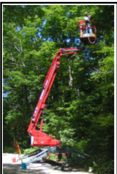
Fig. 2. The dedicated aerial lift for canopy access at HF. The lift design is especially suited for off-road use (Photo: T. Gradowski).
